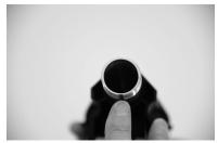
Align the keyway on BUFFER TUBE<sup>(12)</sup> to 6 o'clock position.
