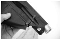
Remove SOCKET HEAD BUTTON SCREWS<sup>(27)</sup> from UPPER STOCK<sup>(1)</sup>.
