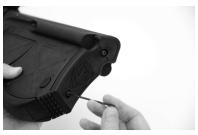
Reattach BUTT PAD(5) and tighten HI-LO SCREWS(20).
