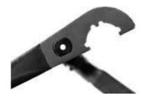
Use your armorer's wrench to engage the cutout at the end of the buffer tube and break it free. Secure the buffer detent with your thumb and continue removing the buffer tube.
