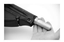
Remove SPACER<sup>(28)</sup> from the BUFFER TUBE<sup>(12)</sup> by tilting UPPER STOCK<sup>(1)</sup> downward and allowing the spacer to slide out.
