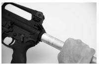
Thread BUFFER TUBE<sup>(12)</sup> onto your firearm while depressing buffer detent until buffer tube secures the buffer detent. Tighten buffer tube to manufacturer's torque specifications. (usually between 30 and 40 ft. lb.)
