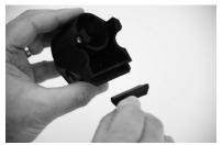
Remove BUMPER<sup>(29)</sup> and install on tapered nose cone.
