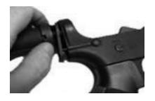
After loosening the castle nut, the end plate disengages, allowing you to unscrew the buffer tube by hand. Pay attention not to lose spring and buffer detent that is secured in place by the end plate.
