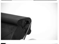
Once **""MULE** ADAPTIVE STORAGE STOCK" is flush with your firearm's lower receiver, secure with SOCKET HEAD CAP SCREW(6).
