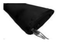
Remove the top butt stock screw.
