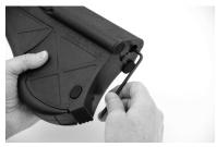
Remove SOCKET HEAD CAP SCREW<sup>(6)</sup> from UPPER STOCK<sup>(1)</sup>.
