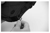
Remove HI-LO SCREWS $^{(20)}$  from BUTT PAD $^{(5)}$  and then remove the butt pad.
