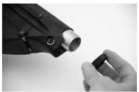
Remove LOCK RING<sup>(19)</sup> from BUFFER TUBE<sup>(12)</sup>.
