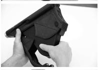
Grasp the MODULE $^{(16)}$  and slide upward along the dovetail rails.
