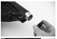
Remove LOCK RING<sup>(19)</sup> from BUFFER TUBE<sup>(12)</sup>.
