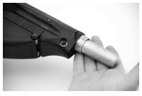
Remove SPACER<sup>(28)</sup> from BUFFER TUBE<sup>(12)</sup> by tilting UPPER STOCK<sup>(1)</sup> downward and allowing the spacer to slide out.
